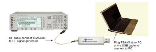
**Figure 9 System Connection**
